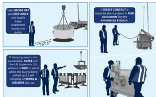
Fig 4 – Unsafe positioning for use of tagline
