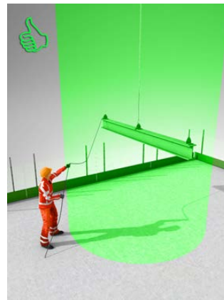
Fig 3 – Correct use of tag line
